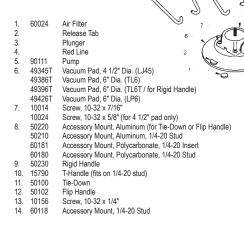
15. 60116 Handi-Grip Handle (for 3" x 6" pad) 50205 Handi-Grip Handle (for 4 1/2" and 6" pads) 16 49365T Vacuum Pad, 3" x 6" (RF36) Vacuum Pad, 3" Dia. (TL3) 17. 49326T 18. 10008 Screw, 10-32 x 3/8" Not Shown 28675 Wood's Powr-Grip® Vacuum Cup Cleaner 29306MM Pad Cover. 3" Pad Cover, 4 1/2"
