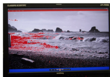
LUM Coloring with All Legal Levels Shown in Greyscale Underexposed Areas in Blue Overexposed Areas in Red
