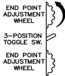
3. BEGIN ROTATING THE WHEEL THAT THE SWITCH WAS PRESSED TOWARDS. THE MOTOR WILL BEGIN TURNING THE LENS. CONTINUE TURNING THE WHEEL UNTIL THE LENS JUST REACHES THE DESIRED STOPPING POINT (EITHER THE END OF LENS TRAVEL OR A DESIRED MARK).
