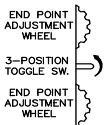
6. RETURN THE TOGGLE SWITCH TO THE CENTER POSITION. TURN THE TRANSMITTER ON. ROTATING THE KNOB (OR MOVING THE SLIDER) END TO END ON THE TRANSMITTER SHOULD CAUSE THE LENS TO MOVE FROM ONE END POINT TO THE OTHER END POINT. IF THE DIRECTION OF LENS ROTATION IS THE OPPOSITE OF WHAT IS DESIRED, SET THE FORWARD/REVERSE TOGGLE SWITCH ON THE TRANSMITTER TO ITS OTHER POSITION.
