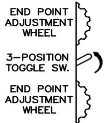
2. PRESS THE TOGGLE SWITCH TOWARDS ONE OF THE WHEELS. THE LENS DRIVE MOTOR WILL MOVE TO THE CENTER OF ITS RANGE OF TRAVEL. ROTATE THE LENS TO THE CENTER OF THE DESIRED RANGE OF TRAVEL AND INTERLOCK THE MOTOR TO THE LENS.
