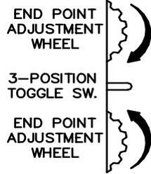
1. WITH THE TRANSMITTER OFF, THE LENS DRIVE MOTOR NOT INTERLOCKED WITH THE LENS, AND THE TOGGLE SWITCH IN CENTER POSITION, ROLL BOTH WHEELS TOWARD THE TOGGLE SWITCH AS FAR AS THEY WILL GO.
