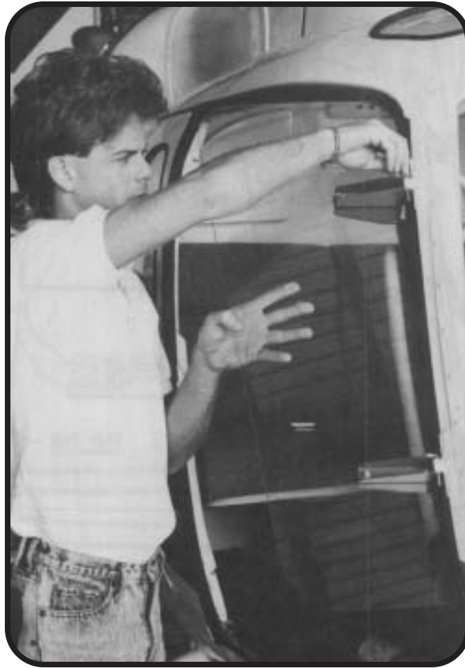
FIG. 11 - Wind-screen installation Right Side View
